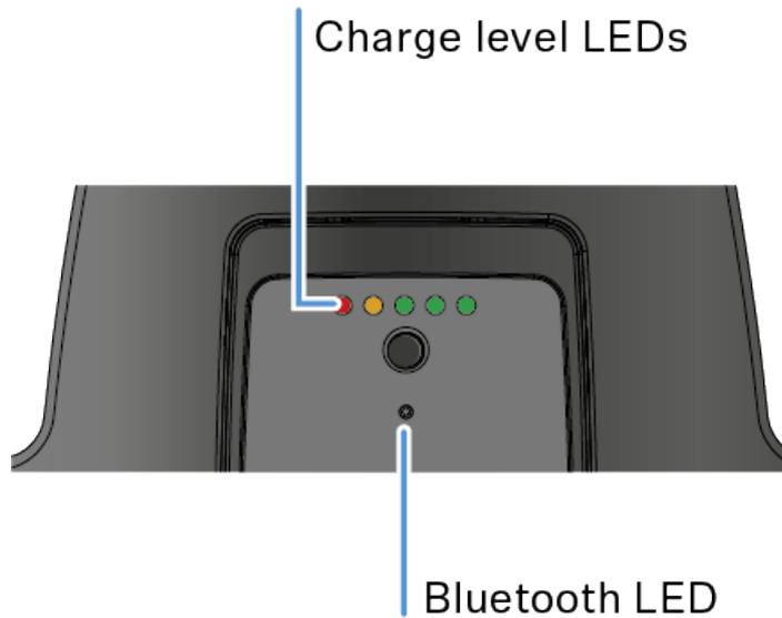
The **charge level** and **Bluetooth** LEDs on the top of the transmitter can indicate the following information.
