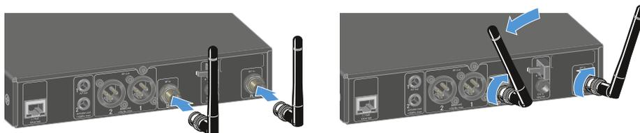
**i** If you are using more than one receiver, we recommend using remote antennas and possibly the [EW-D ASA antenna splitter](#) ([EW-D ASA antenna splitter](#)).
