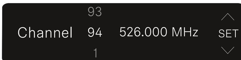
▷ Press the **UP** or **DOWN** button to select a preset channel.
