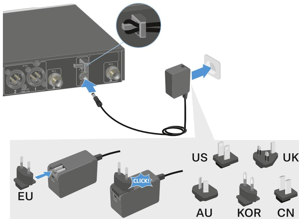
**To completely disconnect the receiver from the power supply system:**
