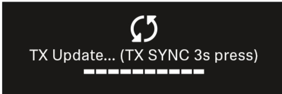
▷ Press the **SYNC** button on the connected transmitter for 3 seconds.
