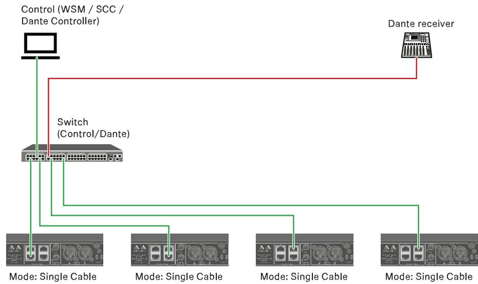
**i** The cable can be connected to network connections I, II or III.
