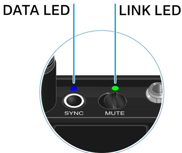
The **LINK** and **DATA** LEDs on the top of the transmitter can indicate the following information.
