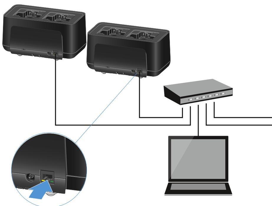
You can integrate the devices into the network individually or cascade up to 5 chargers (see [Cascading chargers](#)).
