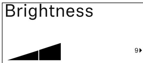
In this menu item, you can adjust the brightness of the transmitter's display.
