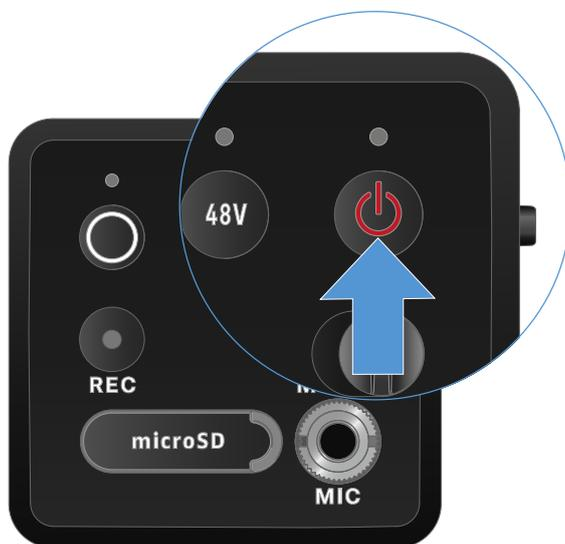
To switch the plug-on transmitter off:
