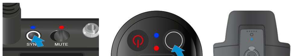
✓ The transmitter and receiver will be synchronized.
