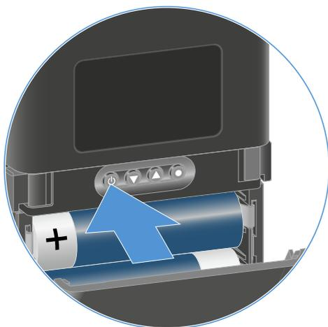
To switch the bodypack transmitter off:
