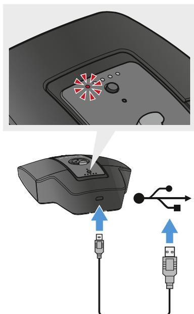
➔ The charge level LEDs indicate the charge level.
