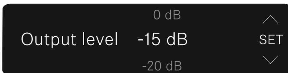
▷ Press the **UP** or **DOWN** button to adjust the value.
