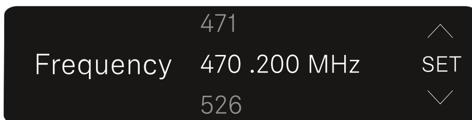
▷ Press the **UP** or **DOWN** button to set the frequency in the megahertz range.
