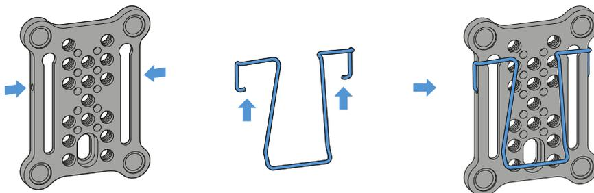
As an alternative to the hot shoe adapter, a metal clip can be attached to the side of the mounting plate.
