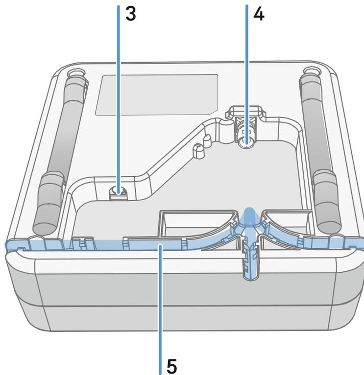
**3 DC in** connection socket for the power supply unit
