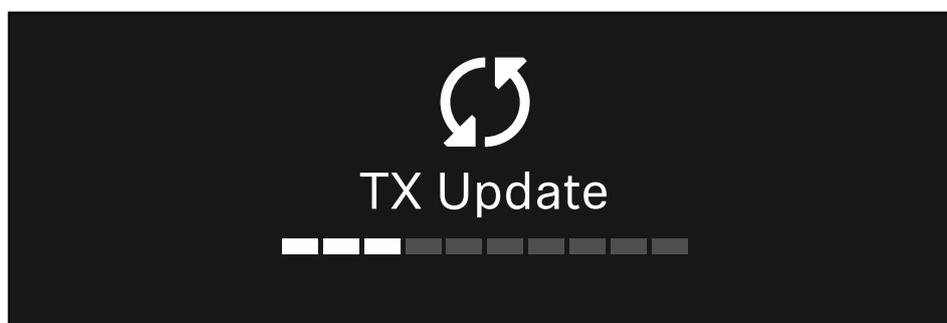
The transmitter's display shows that the firmware update is in progress.
