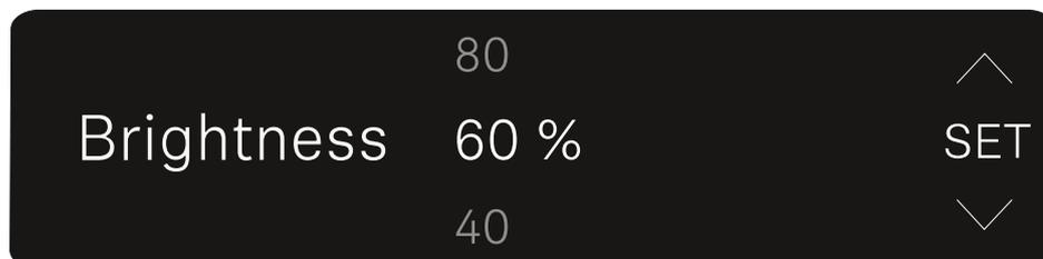
▷ Press the **UP** or **DOWN** button to set the desired brightness.
