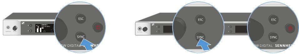
➔ The receiver's display shows that the synchronization process has started.
