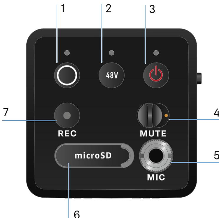
**1 SYNC** button for synchronizing the transmitter and receiver
